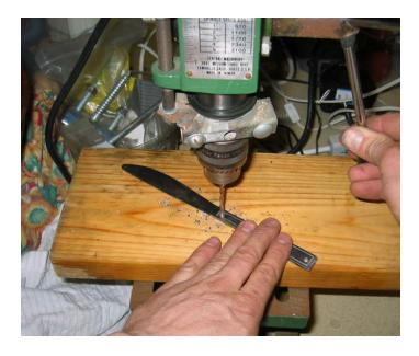
Step 2: Optional: Countersink and Smooth the Holes I'm using a countersink and some sandpaper to do that.
